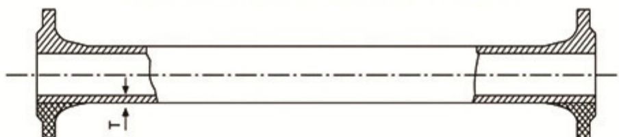
pipes with integrally cast flanges
