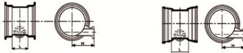
Double-socket level invert with flanged branch
